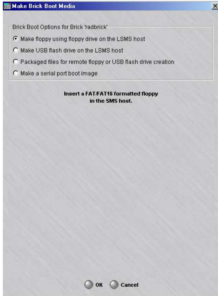
Figure 3-23 Make Brick Boot Media Window
